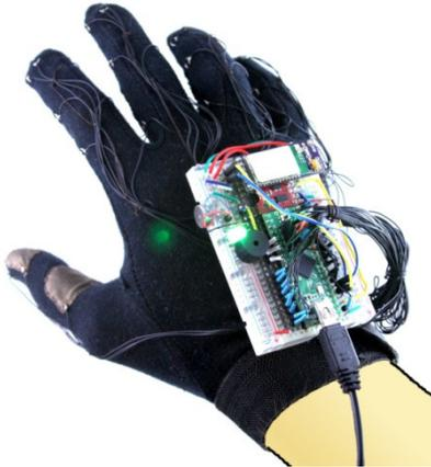
Built using established and well-documented components starting with Atmel's AVR series of microcontrollers, the Keyglove combines conductive fabric and digital motion sensors to detect fingertip touches and both linear and rotational hand motions. The main controller module translates this information into computer control signals, which are then sent to the host computer as HID commands or optionally sent over wired or wireless UART port for completely customized behavior.
